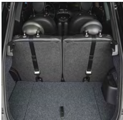
Rear Seat Tether Strap Mounting
