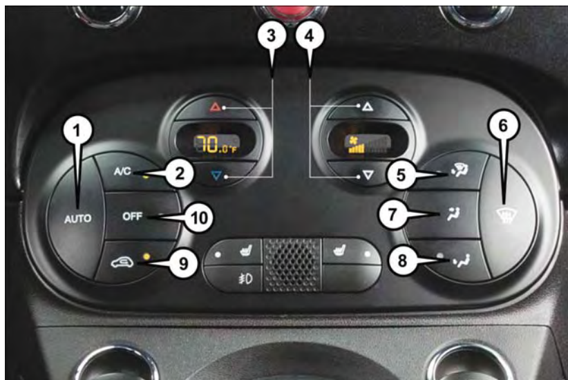
Automatic Temperature Controls
