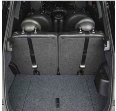
Rear Seat Tether Strap Mounting
