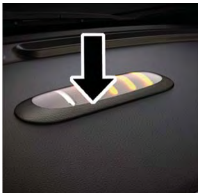
State Of Charge Indicator
