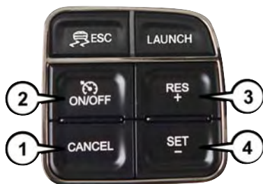
Speed Control Switches
