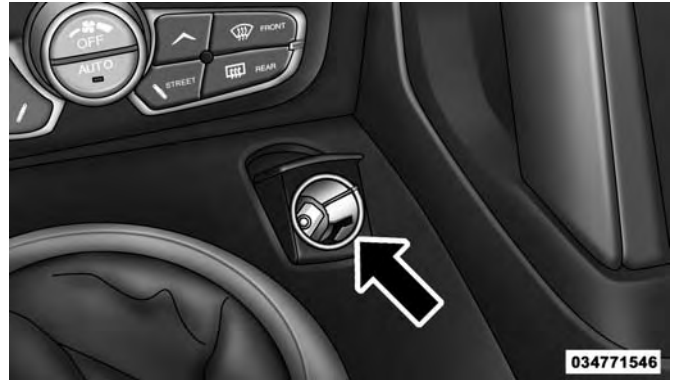
Front Power Outlet
