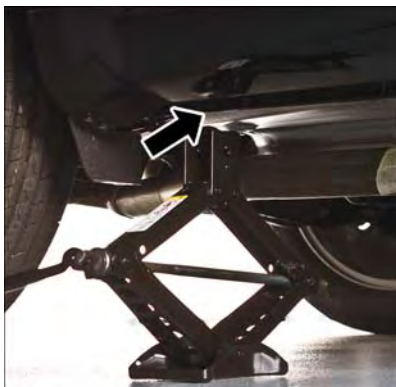
Front Jacking Location
