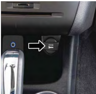
Front Power Outlet
