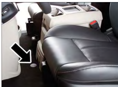
Winch Cover Location
