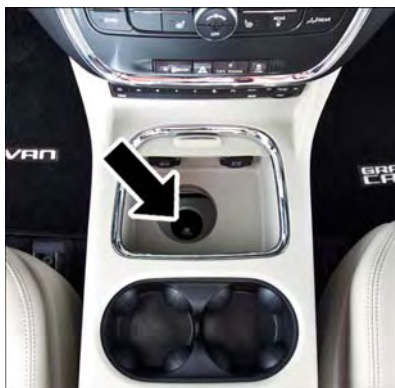
Winch Drive Nut Location
