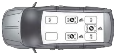
ALR — Switchable Automatic Locking Retractor (2nd Row Quad Seating – Same For Stow 'n Go And Non Stow 'n Go)
