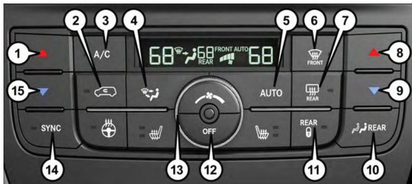
Three Zone Automatic Temperature Controls (ATC)
