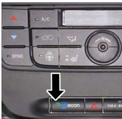
ECON Switch Location
