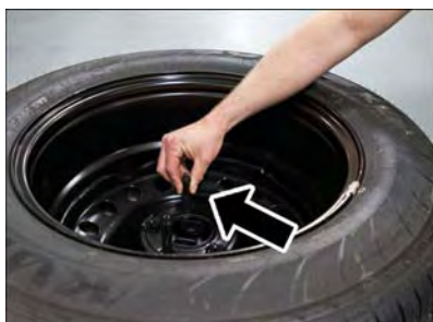
Protective Plate Removal
