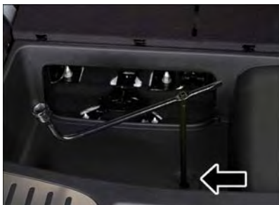
Winch Drive Nut Location
