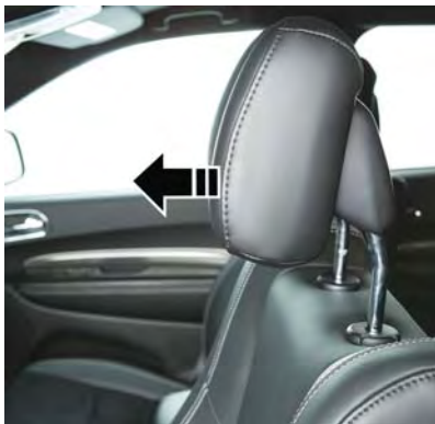
Active Head Restraint (Tilted)
