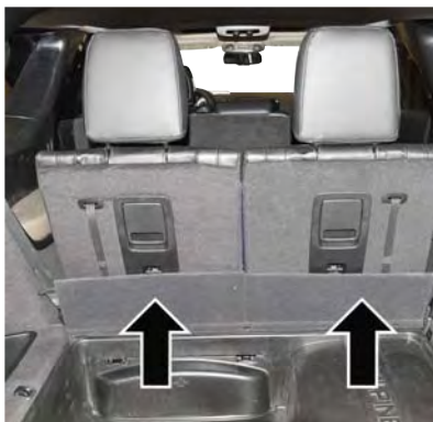
Pulling Down The Carpet Floor Panel To Access Top Tether Strap Anchorage
