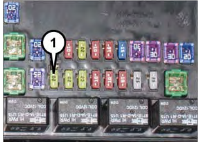
Rear Quarter Power Outlet Fuse
