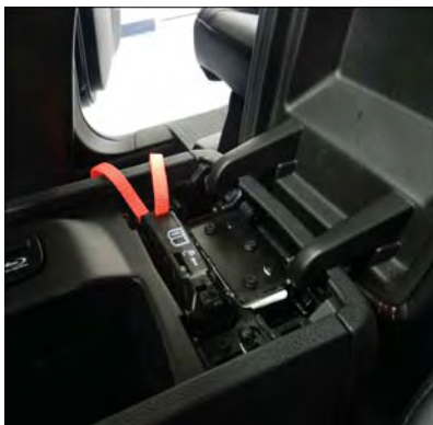
Manual Park Release Cover Removed
