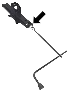
Jack and Tools Assembled
