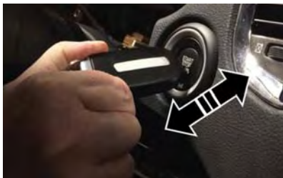
Low Or Dead Key Fob Battery Starting Procedure
