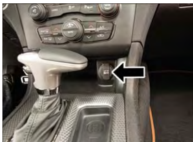
Front Power Outlet
