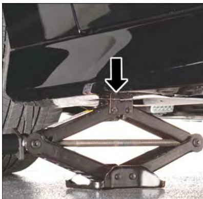
Front Jacking Location
