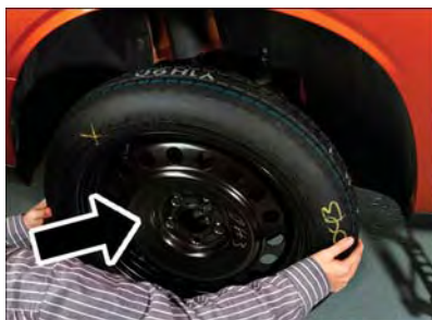
Installing Compact Spare
