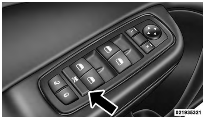
Window Lockout Switch
