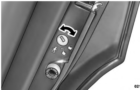
Child-Protection Door Lock Function
