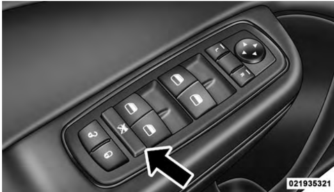
Window Lockout Switch
