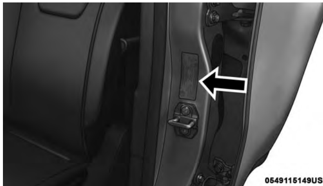
Example Tire Placard Location (B-Pillar)
