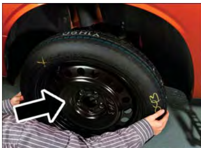
Installing Compact Spare
