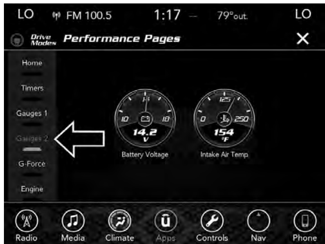
SRT Performance Pages — Gauges 2 (6.4L Manual Transmission)
