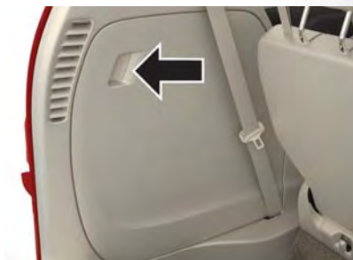
Jacking Equipment Location
