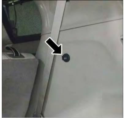
Rear Power Outlet
