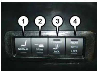
Rear Panel Power Switch Bank
