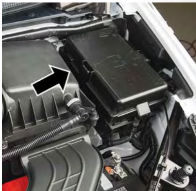
Power Distribution Center
