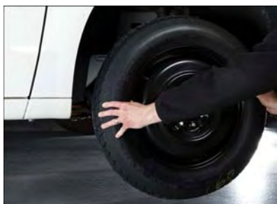
Installing Compact Spare
