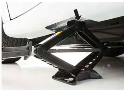
Front Jacking Location Engaged
