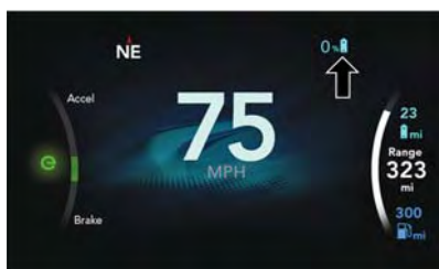
High Voltage Battery Gauge
