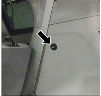
Rear Power Outlet
