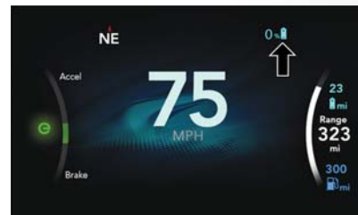
High Voltage Battery Gauge
