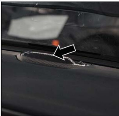
State Of Charge Indicator (Located In The Center Of The Instrument Panel)
