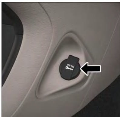
Front Power Outlet
