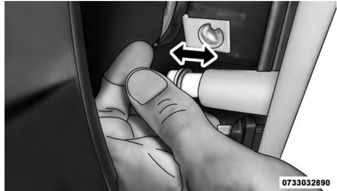
Front Side Marker Lamp Bulb Removal
