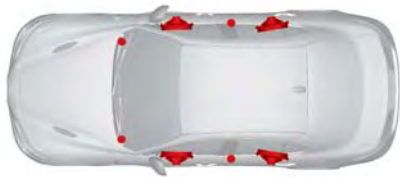
Basic Level Audio System Layout
