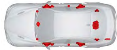
Harman Kardon Premium Audio System Layout
