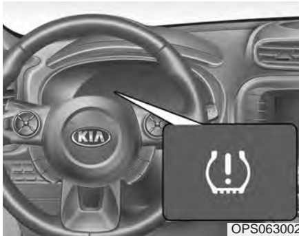
(1) Low tire pressure telltale / TPMS malfunction indicator
