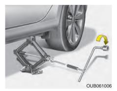
8. Insert the jack handle into the jack and turn it clockwise, raising the vehicle until the tire just clears the ground. This measurement is approximately 1 in (30 mm). Before removing the wheel lug nuts, make sure the vehicle is stable and that there is no chance for movement or slippage.
