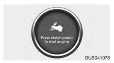
If the engine start/stop button turns to the ACC position twice by pressing the button repeatedly without depressing the clutch pedal, the warning illuminates on the LCD display for about 10 seconds to indicate that you should depress the clutch pedal to start the engine.
