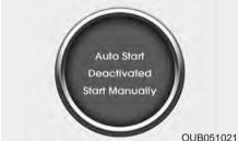
If you open the engine hood in auto stop mode, the light on the ISG OFF button will illuminate and ISG system is deactivated. If your vehicle is equipped with the type B cluster, the notice will illuminate on the LCD display.
