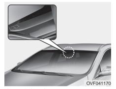
Auto defogging system (Only for automatic climate control system, if equipped)
