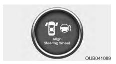
If you start the engine when the steering wheel is turned 90 degrees to the right after a couple of seconds, "Align steering wheel" illuminates on the LCD display for 5 seconds.
