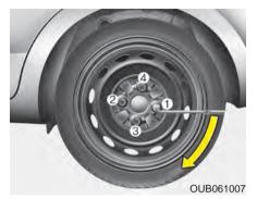
Then position the wrench as shown in the drawing and tighten the wheel nuts. Be sure the socket is seated completely over the nut. Do not stand on the wrench handle or use an extension pipe over the wrench handle.
