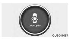
It displays the corresponding door or tailgate that is not closed securely.
