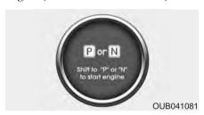
If you try to start the engine with the shift lever not in the P(Park) or N(Neutral) position, the warning illuminates for about 10 seconds on the LCD display.
