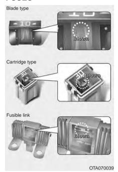
A vehicle's electrical system is protected from electrical overload damage by fuses. This vehicle has 2 fuse panels, one located in the driver's side panel bolster, the other in the engine compartment near the battery.
