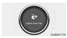
This warning light indicates the fuel filler cap is not tight securely.
