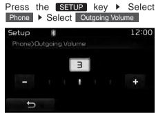
Use the \_\_\_, + buttons to adjust the outgoing volume level.
