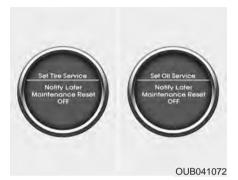
2.If you would like to reset or inactivate the maintenance system press the RESET button for more than 1 second. The display will change to "Engine Oil Service Message" mode.
