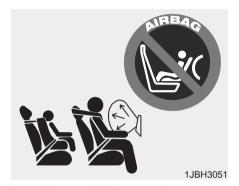
Installing a child restraint on a front passenger's seat is forbidden
