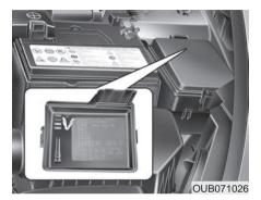
Engine compartment fuse panel
