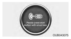
If you press the engine start/stop button while the warning "Key is not detected" is illuminated, the warning "Press the start button with smart key" illuminates for 10 seconds on the LCD display. Also, the immobilizer indicator blinks for 10 seconds
