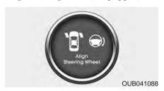
If you start the engine when the steering wheel is turned 90 degrees to the left after a couple of seconds, "Align steering wheel" illuminates on the LCD display for 5 seconds.
