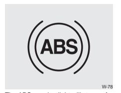
The ABS warning light will stay on for approximately 3 seconds after the ignition switch is ON. During that time, the ABS will go through self-diagnosis and the light will go off if everything is normal. If the light stays on, you may have a problem with your ABS but your regular brakes will work normally. Contact an authorized Kia dealer as soon as possible.
