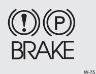
Check the brake warning light by turning the ignition switch ON (do not start the engine). This light will illuminate when the parking brake is applied with the ignition switch in the START or ON position.
