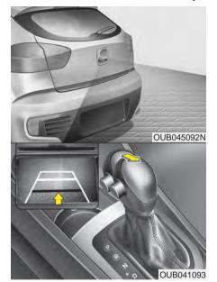
The Rear-Camera Display will activate when the back-up light is ON with the ignition switch ON and the shift lever in the R (Reverse) position.
