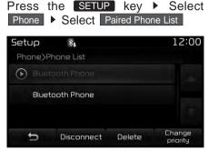
From the paired phone list, select the currently connected device and press the Disconnect button.
