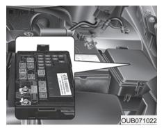
Engine compartment panel fuse replacement
