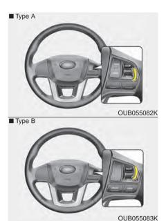
3. Move the lever (1) down (to SET-), and release it at the desired speed. The SET indicator light in the instrument cluster will illuminate. Release the accelerator at the same time. The desired speed will automatically be maintained.
