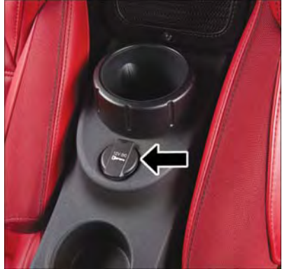
Rear Power Outlet
