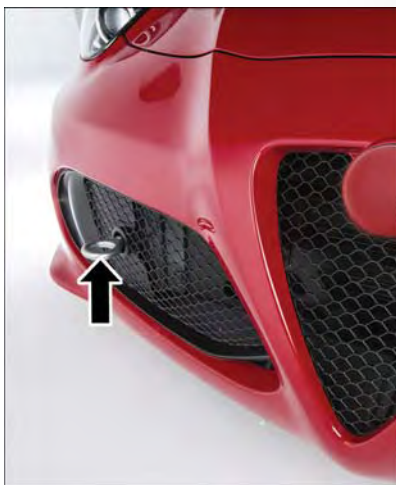
Front Tow Eye Installed
