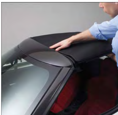
Installing Top Under The Vehicle Spoiler
