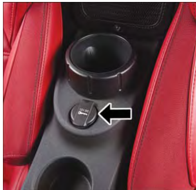
Rear Power Outlet
