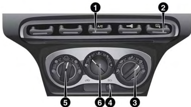
Heating/Ventilation And Air Conditioning Controls
