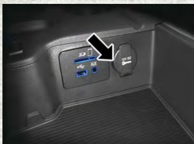
Power Outlet — Storage Compartment
