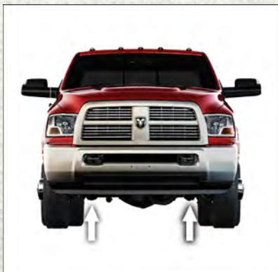
Front Jacking Location
