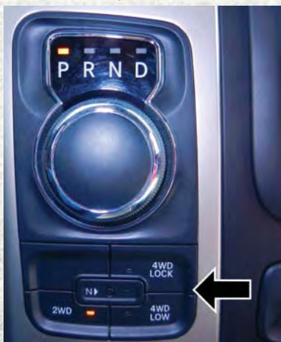
Four-Position/On-Demand Transfer Case — Eight Speed Transmission Only
