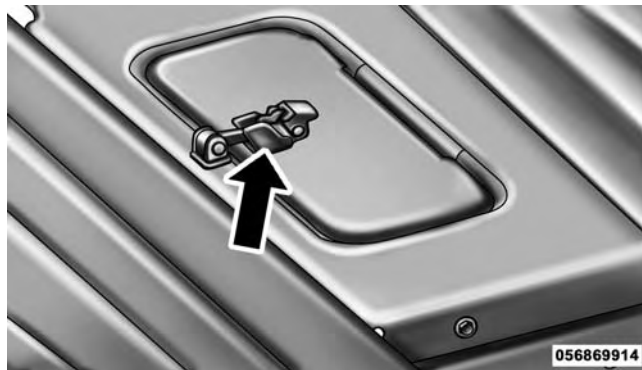
Manual Shut Off Valve Access Door
