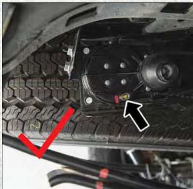
Winch Mechanism Properly Engaged (Yellow DOT Will Appear In The Winch Indication Window)
