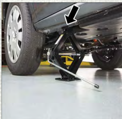
Front Jacking Location Engaged
