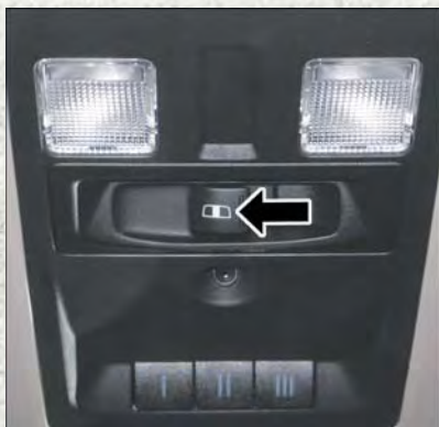
Power Sliding Rear Window Switch
