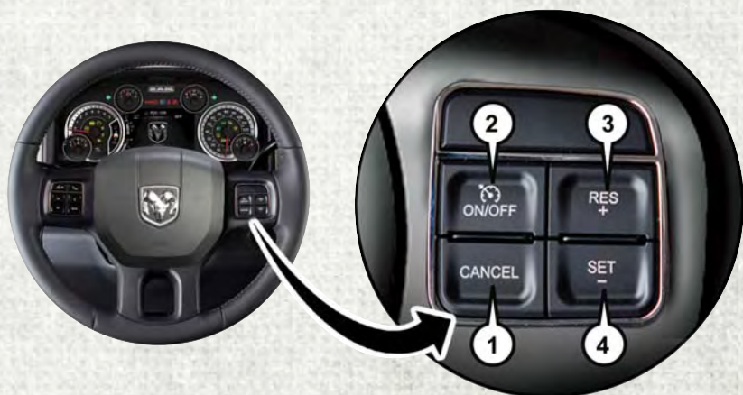
Speed Control Switches
