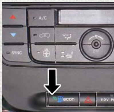
ECON Switch Location
