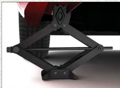
Rear Jacking Location Engaged
