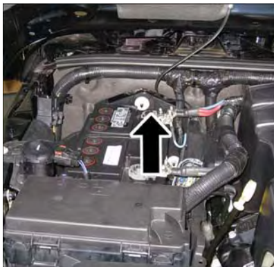
Positive Battery Post
