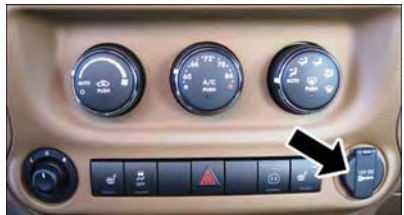
Power Outlet — Front
