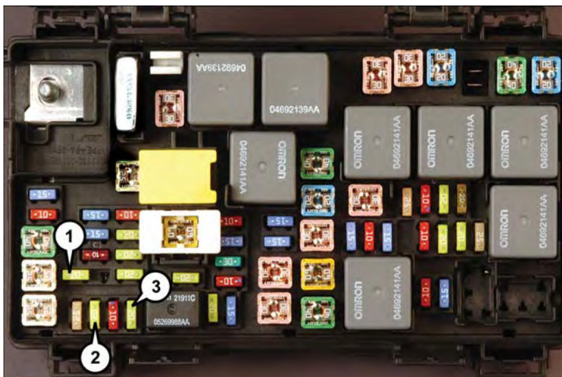
Power Outlet Fuses
