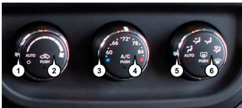
Automatic Temperature Controls
