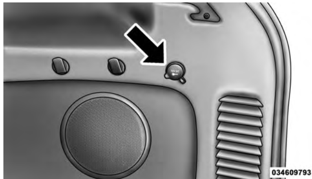
Rear Power Outlet
