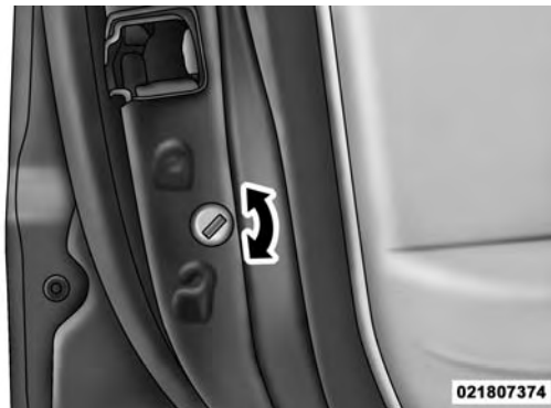
Child-Protection Door Lock Function
