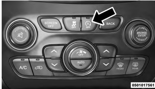
STOP/START OFF Switch
