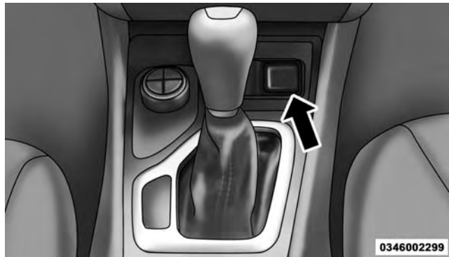
Front Electrical Power Outlet
