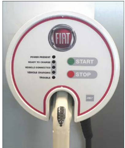
Electric Vehicle Supply Equipment (EVSE)
