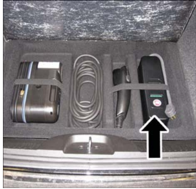
Electric Vehicle Supply Equipment (EVSE)
