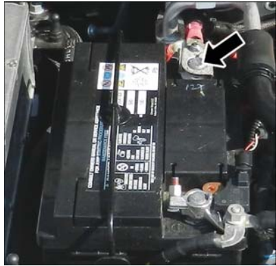
Positive Battery Post
