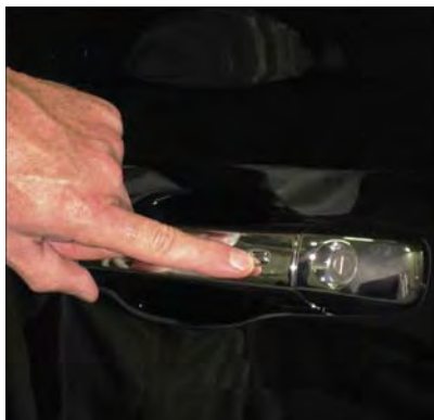
Push The Door Handle Button To Lock
