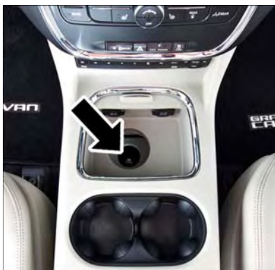
Winch Drive Nut Location
