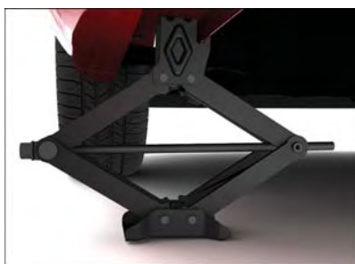
Rear Jacking Location Engaged
