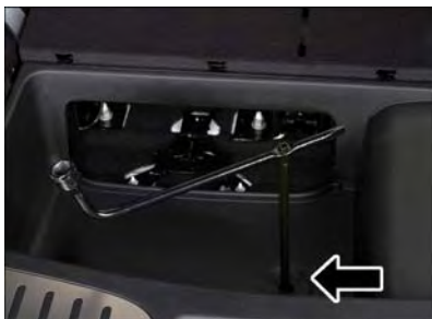
Winch Drive Nut Location
