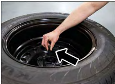
Protective Plate Removal
