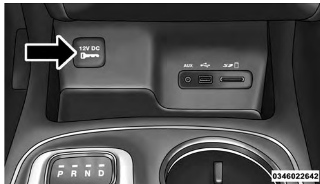
Front Power Outlet
