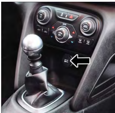
Front Power Outlet
