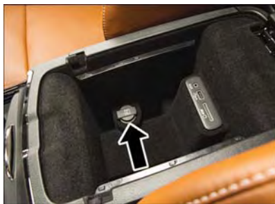
Center Console Power Outlet
