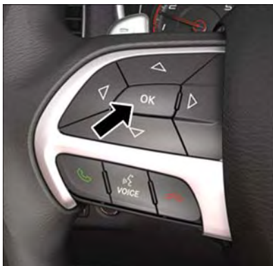
SRT DID Controls
