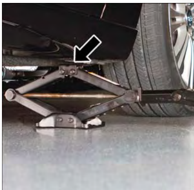
Front Jacking Location
