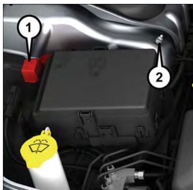
Remote Battery Posts
