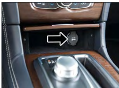
Front Power Outlet
