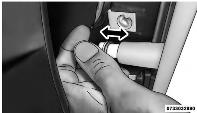
Front Side Marker Lamp Bulb Removal
