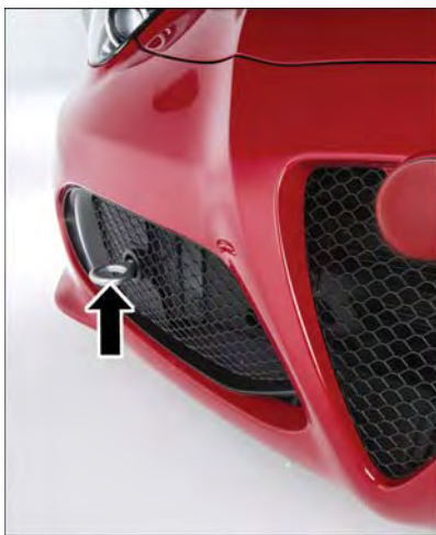
Front Tow Eye Installed
