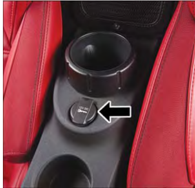
Rear Power Outlet
