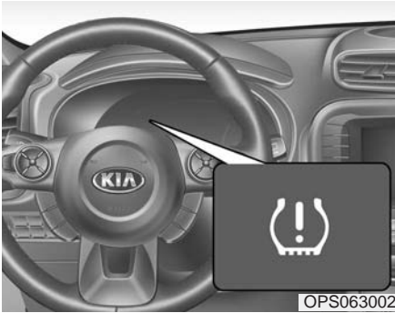
(1) Low tire pressure telltale / TPMS malfunction indicator
