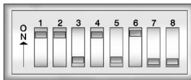
Example of Eight Dip Switches with Two Positions
