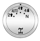
This transfer case knob is located next to the steering column.
