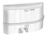
The fluid level should be above MIN. If it is not, have the brake hydraulic system checked to see if there is a leak.
