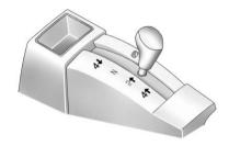
This transfer case shift lever is on the floor to the right of the driver.
