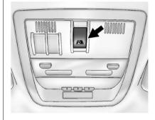
If equipped, the power sliding rear window works when the ignition has been turned to ACC/ACCESSORY or ON/RUN, or when Retained Accessory Power (RAP) is active. See Retained Accessory Power (RAP) on page 9-27.
