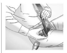
If the belt stops before it reaches the buckle, when using the lap-shoulder belt in a rear center seating position of a crew-cab, tilt the latch plate and keep pulling the safety belt until it can be buckled.
