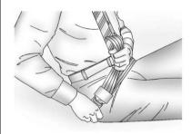
To make the belt shorter, pull its free end as shown until the belt is snug.
