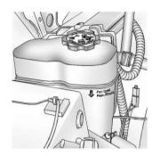
The coolant level should be at or above the FULL COLD mark. If it is not, there may be a leak in the cooling system.
