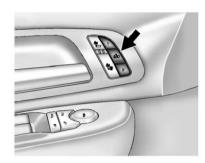
If available, the controls on the driver door are used to program and recall memory settings for the driver seat, outside mirrors, and the adjustable throttle and brake pedals, if equipped.
