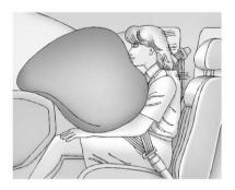
The right front passenger airbag is in the instrument panel on the passenger side.
