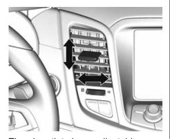
The air outlets have adjustable vanes that move up or down and left or right to change the direction of the airflow. Use the thumbwheels located near the air outlets on the instrument panel to shut off the airflow.
