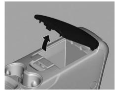
There is storage under the center console armrest. To open, press the latch and lift up. Do not force the lid backwards. There is a power outlet inside.
