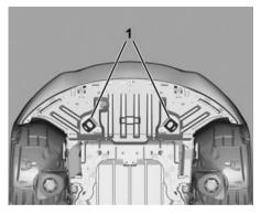
There are 2 oval-shaped slots (1) under the front of the vehicle that should be used to move a disabled vehicle. Use only these slots to hook to the vehicle. The slots can be accessed through the splash shield. Use an appropriate size T hook for the slot.
