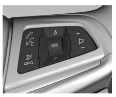
Some audio functions can be controlled through the steering wheel controls.
