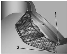
Attach four corner loops (1) to the top two hooks on the vehicle (two loops on one side, two loops on the other) and attach the two center loops (2) to the bottom hooks on the vehicle.
