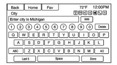
Letters of the alphabet, symbols, punctuation, and numbers, when available, display on the navigation screen as alpha/numeric keyboards. The alpha keyboard displays when data needs to be entered.
