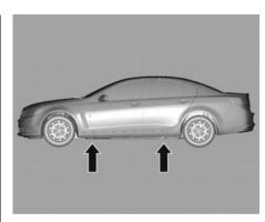
7. Position the jack lift head at the jack location nearest the flat tire. The locations are identified by cutouts in the underside of the door sill. The jack must not be used in any other position.
