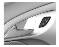
**a** (Unlock): Press to unlock the doors.
