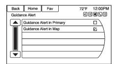
Press to enable the guidance alert pop-up to be viewed on the map or on the main screens such as audio, weather, phone, etc. A checkmark appears to indicate the guidance alert mode is on.
