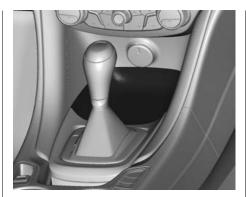
Remove the trim from the center console, in front of the shift lever.
