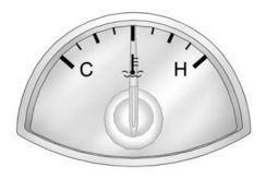
This gauge shows the engine coolant temperature.
