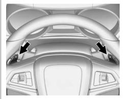
Alternatively, the paddles can be used to shift to the required gear:
