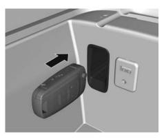
Place the recognized transmitter in the transmitter pocket. The transmitter pocket is inside the center console storage area.
