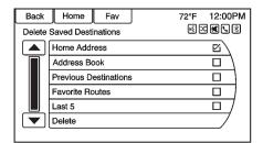
Press to delete all saved destinations. A Delete Saved Destinations submenu displays. Select the desired options for deletion and press delete at the bottom to continue. A confirmation screen displays requesting to delete or cancel.
