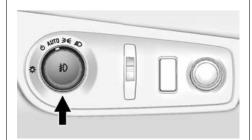
The exterior lamp control is on the instrument panel to the left of the steering wheel.
