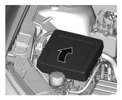
To access the fuse block, remove the clip-on cover.
