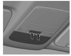
The dome lamps are in the overhead console.
