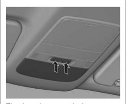
The dome lamps are in the overhead console.
