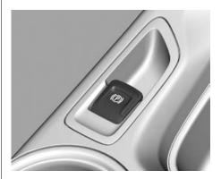
The vehicle has an Electric Parking Brake (EPB). The switch is on the center console. The EPB can always be activated, even if the ignition is off. To prevent draining the battery, avoid repeated cycles of the EPB when the engine is not running.
