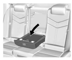
The rear seat has a rear seat pass-through door in the center of the rear seatback. Press the button on top of the seatback and fold the center part of the seatback down to access the trunk. There are two cupholders on the door. To close, lift the pass-through door and push it rearward until it locks into place.
