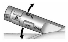
Move the turn signal lever all the way up or down to signal a turn.
