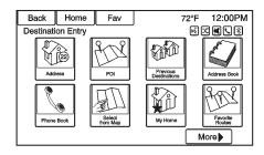
If route guidance is not active, press the Destination screen button on the Home Page to access the Destination Entry screen. Several options can be selected to plan a route by entering destinations.
