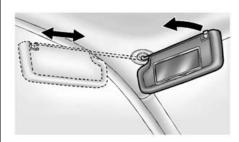
Pull the sun visor down to block glare. If equipped, detach the sun visor from the center mount to pivot to the side window or to extend along the rod.
