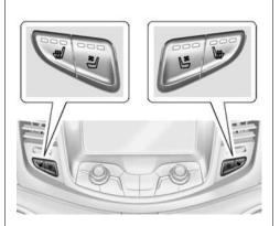
The buttons are below the air vents on the center stack. To operate, the engine must be running.
