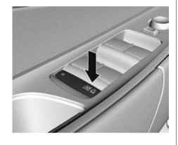
Press to prevent rear seat passengers from operating the windows. The indicator light illuminates when on. Press again to turn the feature off. This also activates the safety locks on the rear passenger doors.
