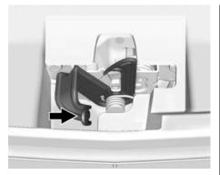
2. Push up on the secondary hood release and lift the hood.
