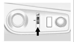
This feature controls the brightness of the instrument panel controls and infotainment display screen. The thumbwheel is to the left of the steering column on the instrument panel.
