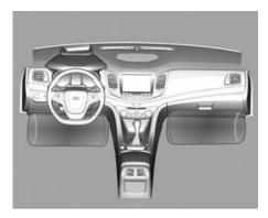
The driver knee airbag is below the steering column. The front outboard passenger knee airbag is below the glove box.
