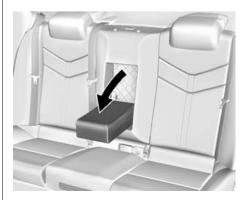
The rear seat has an armrest in the center of the seatback. Pull the armrest down to lower it. To fold, lift the armrest up and push it rearward until it is flush with the seatback.
