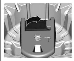
The tire sealant and air compressor kit is located in a foam container in the trunk, under the floor carpet.
