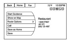
**Start Guidance:** Press to start route calculation to the destination(s) received.
