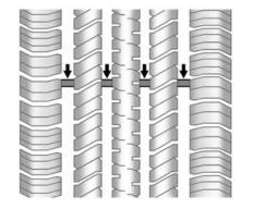
Treadwear indicators are one way to tell when it is time for new tires. Treadwear indicators appear when the tires have only 1.6 mm (1/16 in) or less of tread remaining. See *Tire Inspection on page 10-46* and *Tire Rotation on page 10-47*.
