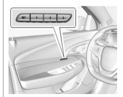
The SET, "1," "2," and "3" buttons on the driver door are used to manually save and recall memory settings for the driver seat and outside mirrors. These manually stored positions are referred to as Button Memory positions.
