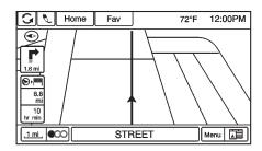
The Menu screen button at the bottom right side of the display accesses the Navigation Menu.
