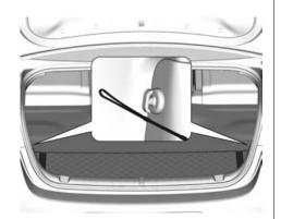
If equipped, the convenience net is in the rear. Put small loads behind the net. It can also be positioned into an envelope style to hold smaller items. The net is not for heavier loads. Store items as far forward as you can.
