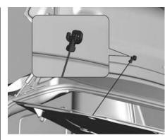
2. Lift the cover with the handle/ strap and attach the hook to the trunk lid.
