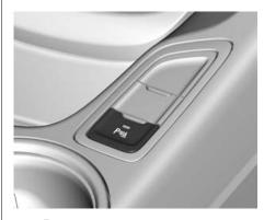
The PM button near the shift lever is used to turn on or off the Front and Rear Parking Assist. The indicator light next to the button comes on when the features are on and turns off when the features have been disabled.
