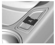
The system is available when the vehicle speed is below 30 km/h (18 mph). Press Pont to enable the system to begin searching for a space that is large enough to park. The system cannot detect whether it is a legal parking space.
