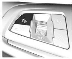
The Collision Alert control is on the steering wheel. Press to set the FCA timing to Far, Medium, Near, or Off. The first button press shows the current setting on the Head-Up Display (HUD). Additional button presses will change this setting. The chosen setting will remain until it is changed and will affect the timing of both the Collision Alert and the Tailgating Alert features. The timing of both alerts will vary based on vehicle speed. The faster the vehicle speed, the farther away the
