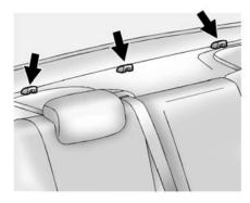
The top tether anchors are on the rear seatback filler panel. Be sure to use an anchor on the same side of the vehicle as the seating position where the child restraint will be placed.
