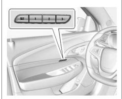
The SET, "1," "2," and "3" buttons on the driver door are used to manually save and recall memory settings for the driver seat and outside mirrors. These manually stored positions are referred to as Button Memory positions.
