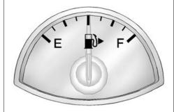
When the ignition is on, the fuel gauge shows how much fuel is left in the fuel tank. When the indicator nears empty, a message in the Driver Information Center (DIC) displays. See *Fuel System Messages on page 5-28*. The vehicle still has a little fuel left, but the vehicle should be fueled soon. An arrow on the fuel gauge indicates the side of the vehicle the fuel door is on.
