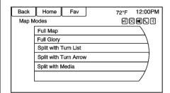
Press to change the view of the maps while using the navigation function. The system offers a variety of full and split views. Some views are only selectable when route guidance is active.
