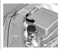
Turn the coolant recovery reservoir dipstick cap counterclockwise and slowly pull out the dipstick. There are maximum and minimum markings on the dipstick.
