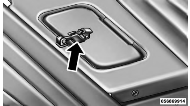
Manual Shut Off Valve Access Door
