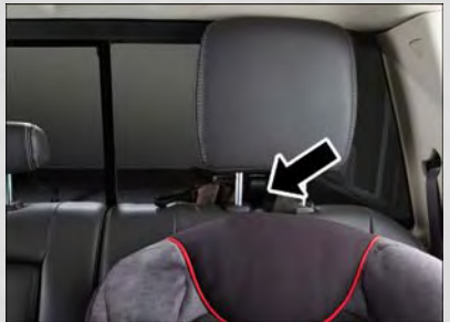
Tether Strap Through Outboard Tether Strap Loop
