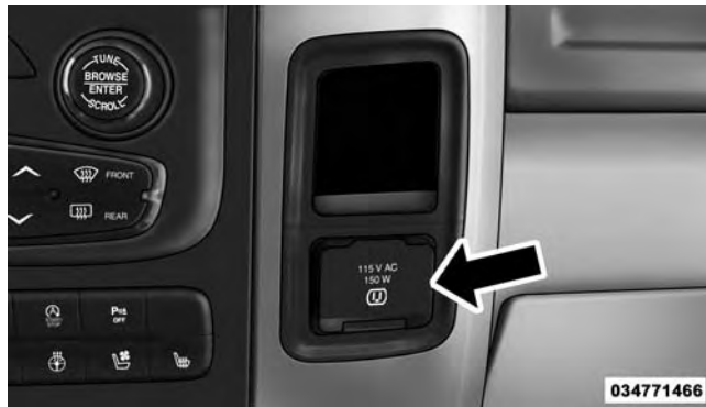
Power Inverter Outlet
