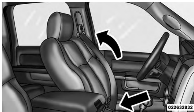
Removing Slack From Belt
