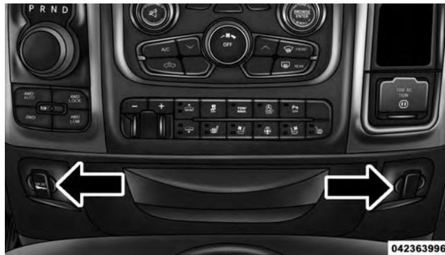
Power Outlets — Center Stack
