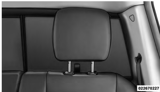
Head Restraint In Raised Position
