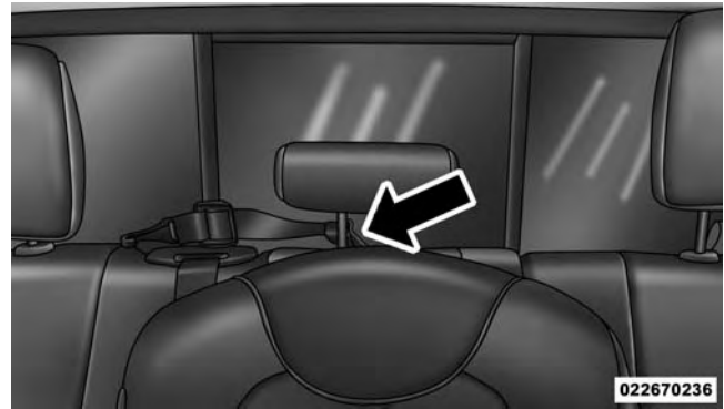
Tether Strap Through Center Tether Strap Loop
