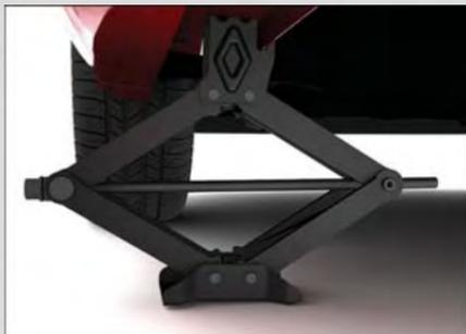
Front jack location is on the sill flange of the vehicle body and is located 6 in (150 mm) from door edge.
