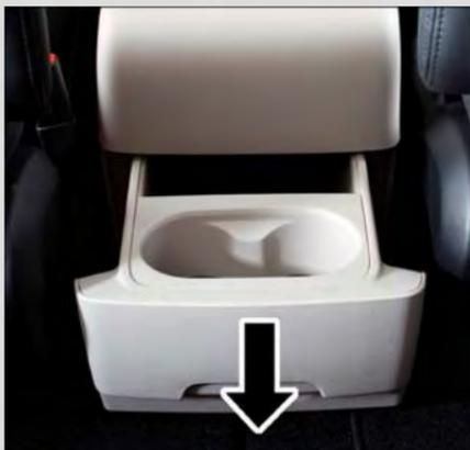
3. Remove the liner from the console's storage compartment to access the spare tire winch drive nut.
